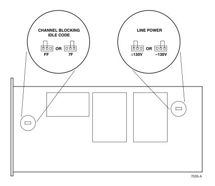
Figure 525-3. Placement of B2 RLX+ Jumpers
